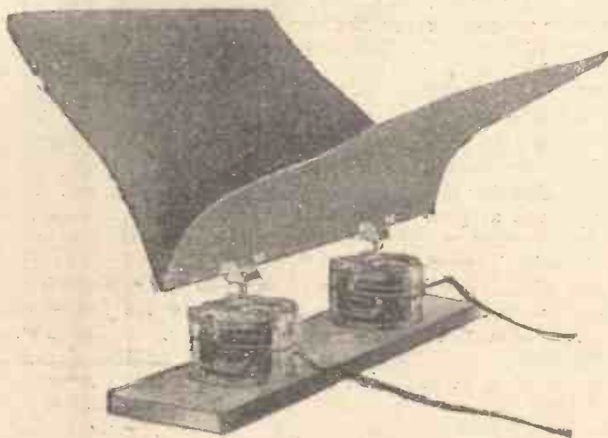
This is how the two units and the diaphragm are arranged
