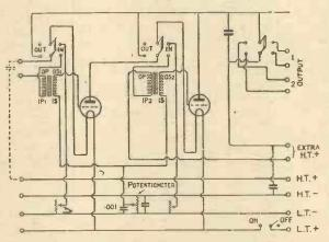
Fig. 1.-Circuit Diagram of Note-magnifier Unit.
