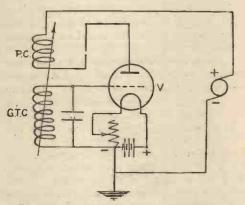
Diagram of Simple Transmitting Circuit.
