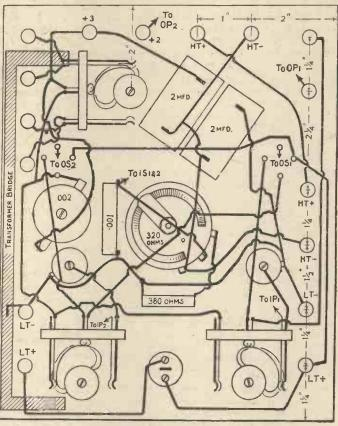
Fig. 2 .--- Wiring Diagram of Note-magnifier Unit.
