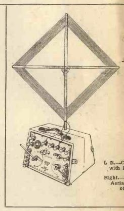
short, it is desirable to use one turn of wire enclosing a large area rather than more turns enclosing a smaller area.
