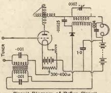
Circuit Diagram of Reflex Circuit.
