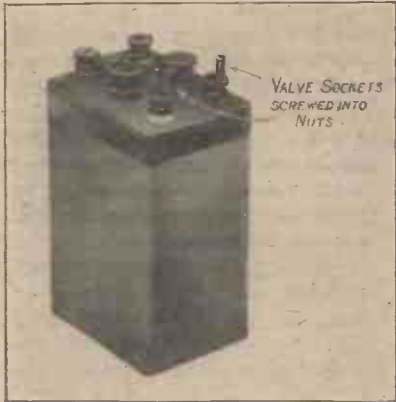
Fig. 10.—Photograph of Accumulator with Valve Sockets Fitted to Terminals.
