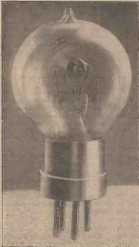
An Ordinary Type of Thermionic Valve or Triode and its Component Parts.
