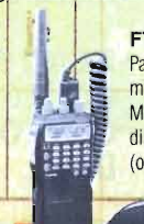
FT 51 R Palmare bibanda VHF/UHF, Rx: 370/480 MHz; 800/999 MHz; 110/174 MHz e banda aeronautica (110/138 MHz in AM) 120 memorie.
