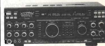
YAESU FT-1000/FT-990 2 VFO - 100 kHz - 30 MHz - All Mode - 100 memorie - 200 W RF (FT 990 100 W RF).
