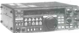
TS 711 E/DCS VHF 144-146 MHz TS 811 E/DCS UHF 430-440 MHz 2 m, 25 W, All Mode base. 70 cm, 25 W, All Mode base.
