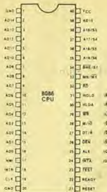
MAXIMUM MODE PIN FUNCTIONS IN G. (20P) ARE SHOWN IN PARENTHESES
