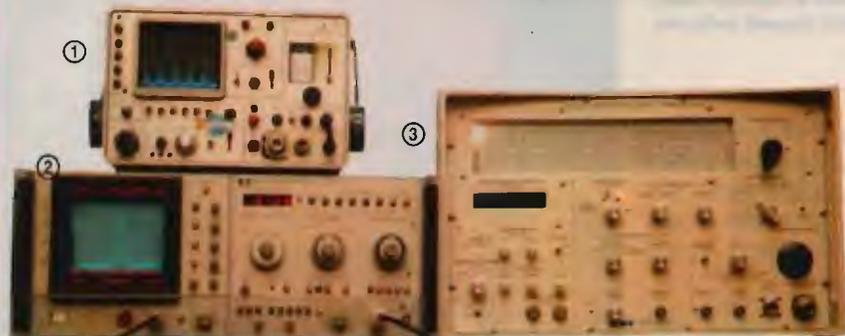
① Spectrum Analyzer, TEK 491 • ② Spectrum Analyzer, HP 8565A • ③ Kay-1520A, 0,05-1200 MHz.
