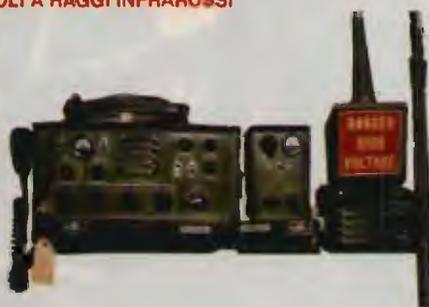
RTX, SSB/AM/CW, RT 902 - 2 ÷ 15 MHz, con Ant-coupler CU 1782.
