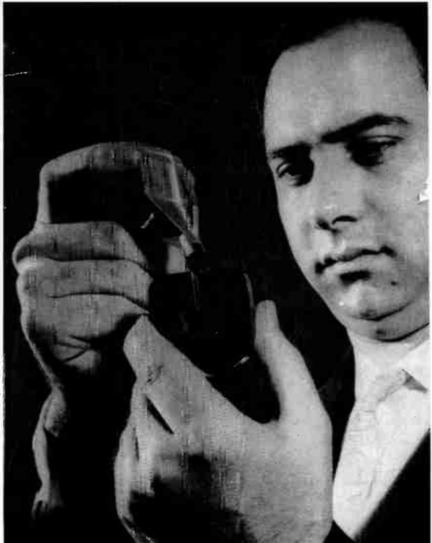
Half-inch square crystal of synthetic ruby at tip of copper transition section is held above a 12-ounce magnet to dramatize the "heart" of the revolutionary "ruby maser" developed by Hughes Aircraft for the U.S. Army Signal Corps.
