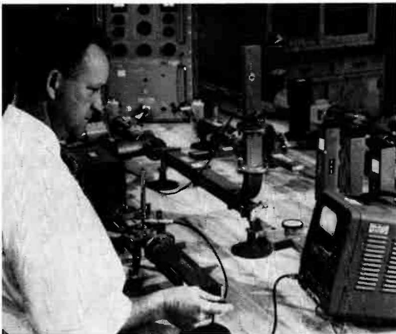
Laboratory engineer in the microwave section of Convair is shown making standing wave measurements on radar waveguides with the slotted line technique.
