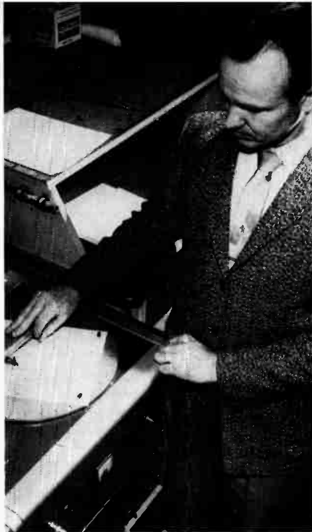
Collins Radio Company engineer is pictured recording a radiation pattern from the bicone antenna to be used in Project Mercury. The Collins Antenna Laboratory is utilizing two full scale models of the Mercury capsule for testing all the antennas.
