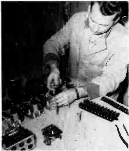
In the assembly shop of Mechtron Engineering Products, a technician assembles and wires a control panel for the No-Break diesel electric power plants for the Air Defense Communication System.
