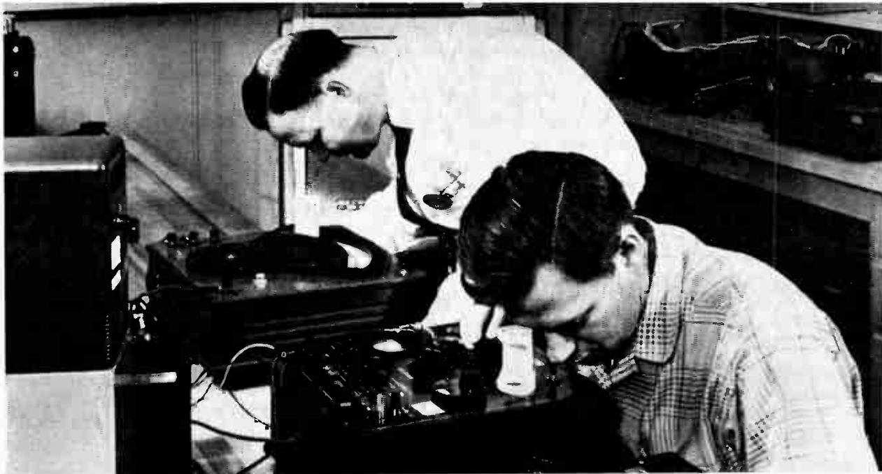
Two members of the Western Primary Standards Laboratory staff at Convair (Pomona) Division of General Dynamics Corporation at Pomona, Calif., compare the performance of a "secondary standard" instrument (center) with the output of the "primary standard" dynamometer (at rear).
