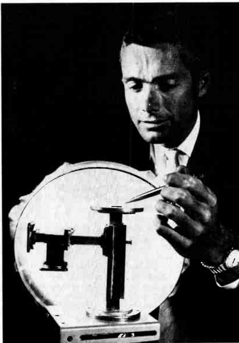
Charles W. Curtiss, manager of Hughes Aircraft Company's microwave engineering department, examines new "parametric amplifier" for use in aircraft and airport radar systems. New amplifier is expected to increase range of both systems by as much as 100 per cent.
