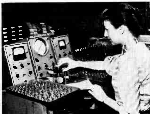
Variable resistors being checked at Precision Electronic Components (1956) Ltd., Toronto, Ontario. The above illustration shows the final inspection in which the taper-noise and the hop-off resistance of L-type variable resistors are checked in one automatic operation.
