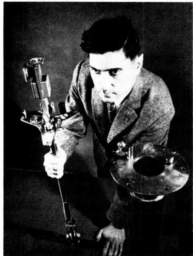
Shown at left above is the complete "ruby maser" weighing only 25 pounds and measuring 30 inches high and five inches in diameter. At right is the Hughes Aircraft Company's maser microwave circuits with an integrated permanent magnet (at bottom). In the foreground is the double coolant container into which the unit is installed to supercool the ruby crystal to a few degrees above absolute zero.
