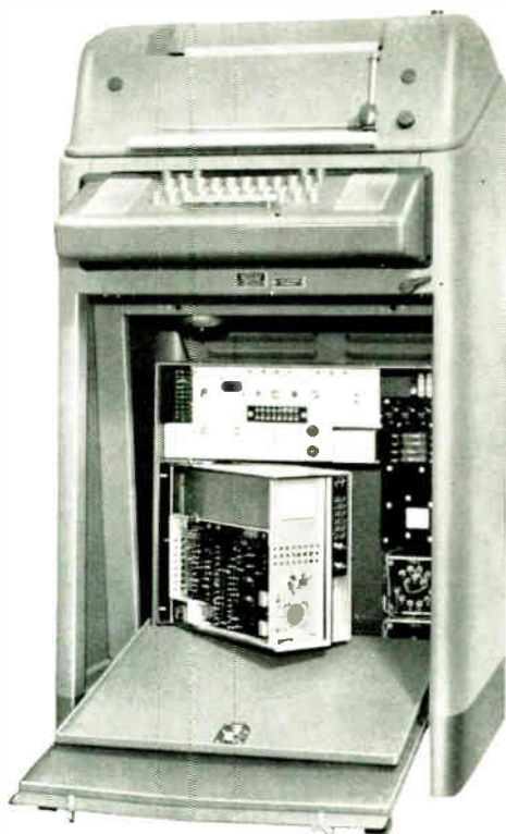
Type 2340A Subscriber Set mounted in the knee-well of a Model 28 Teletypewriter
