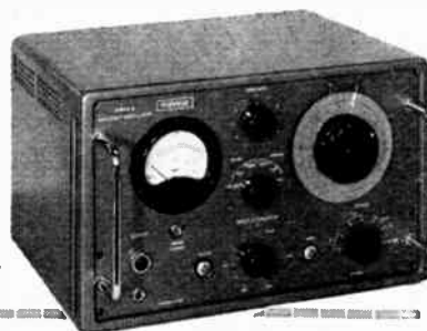
D-888-A (Analyser/Oscillator) Frequency: 200c/s to 650kc/s Accuracy: 2% Output (OSC): 2.5v into 600 ohms
