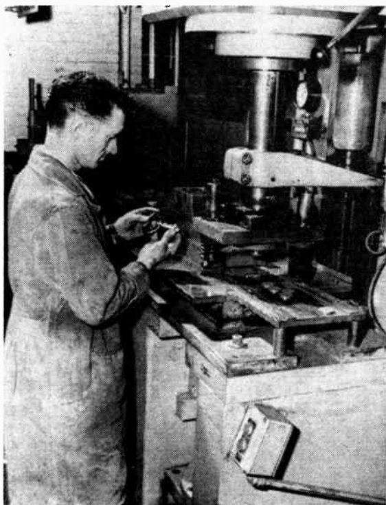
Figure 3. The unit shown at the left is a double ran hydraulic press of 50 ton capacity used for pressing ferrite parts. The action is completely automatic and a rate of 600 parts per hour can be achieved in a single cavity tool.
