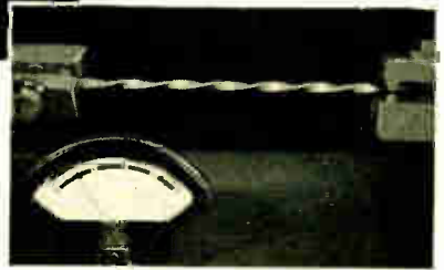
Twist test shows insulation adhering firmly to the copper while wire is being subjected to extreme torsion.
