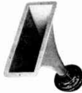
RP-103 HORN TWEETER Magnet — 4.64 oz. Voice Coil — 16 ohms, 1" diameter. Cycles — 2,000 to 20,000.
