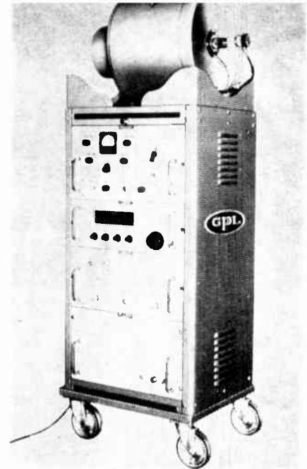
● New Model PB-611A television projection system developed by General Precision Laboratory of Pleasantville, N.Y. The portable unit incorporates a newly designed optical system which greatly increases light output over earlier designs.
