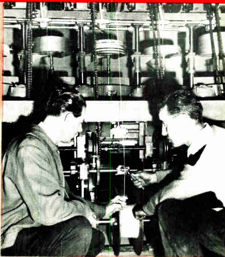
WINNIPEG WORKER GAINS NEW SKILL: John Hodge (above right) learns the intricate job of insulating copper wire with strip paper on a new five-head machine being installed at the Telecables & Wires Ltd. plant at Fort Garry, Manitoba. Instructor Vic Wilson, from the Canada Wire and Cable Company Limited plant at Leaside, Toronto, shows him the proper technique. Canada Wire is part owner of the new Telecables plant and operates it under a management contract. The plant is the first communications cable manufacturing unit in Western Canada.
