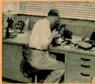
Microscopic and petrographic equipment used in Ohmite laboratories for optical examination of materials and products.
