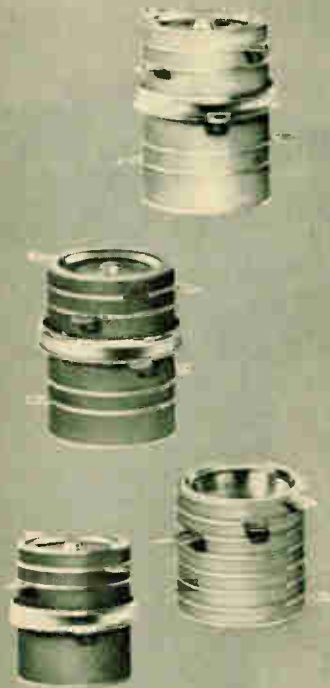
New stacked ceramic receiving tubes that can withstand heavy shock and vibration
