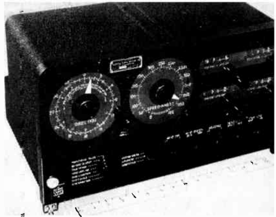
● Course and Position Indicator displays data used in airborne navigation and continuously indicates present position of aircraft in latitude and longitude. The Indicator is a vital part of the complete AN/APN-66 global Navigation Systems.
