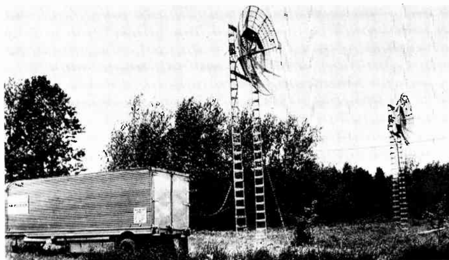
● The Kingmere, Quebec, installation of the Scatter Propagation demonstration of the Collins Radio Company of Canada. The second installation was located 120 miles distant about 15 miles south of Montreal.
