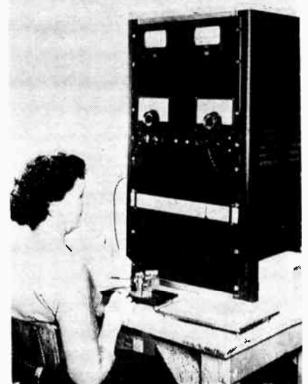
● The above photograph shows the "K" gage being used in a mica splitting operation.
