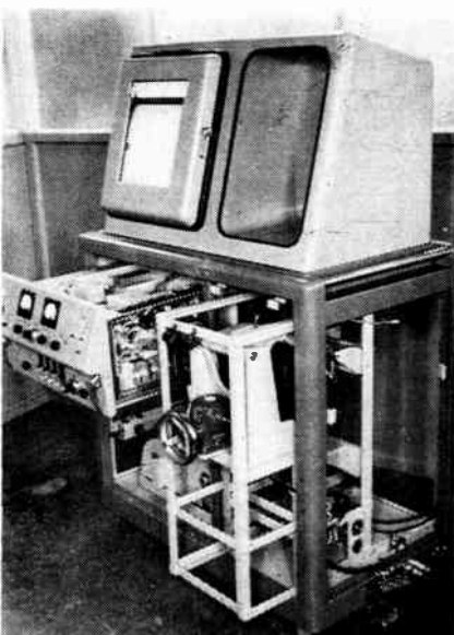
● Left: The Consolidated Type 21-610 "Process Monitor" Mass Spectrometer with side panels removed to show unit construction. All electronics circuits are contained in the "electronics drawer" in upper left of cabinet. The combination recorder-and-inlet-system housing on top of cabinet is an accessory. Right: Consolidated Electro-dynamics' Analytical Mass Spectrometer, showing (l. to r.) inlet cabinet with micromanometer, the magnet and its pedestal, and control console. The recording oscillograph is in the upper left hand corner of the console.
