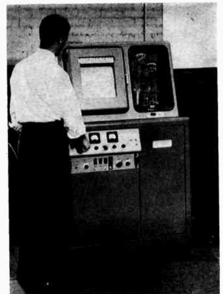
● Left: Taking samples at the sulphur recovery plant. Minute quantities of the sample taken were fed to the inlet system of the Consolidated 21-610 Process Monitor Mass Spectrometer installed in the mobile laboratory. Right: The Consolidated Type 21-610 "Process Monitor" Mass Spectrometer.
