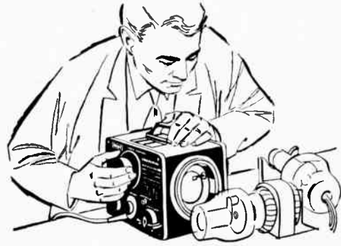
Checking a rotating anode X-ray tube for acceleration and smooth operation in a matter of minutes, with a Dawe Stroboscope.
