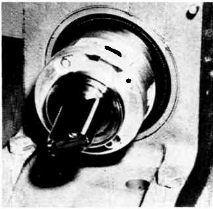
● Compound headstock permits aligning proper crystallographic plane to cutting plane of saw. Shown here is a germanium crystal cemented to headstock and aligned in proper plane.
