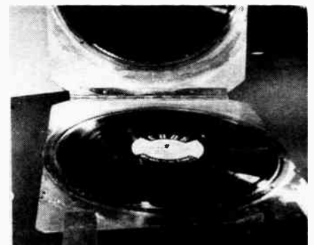
Left: Pure vinyl "Biscuit" formed by gentle heating of the powder. Center: Biscuit in press with label applied. Right: Completed record.
