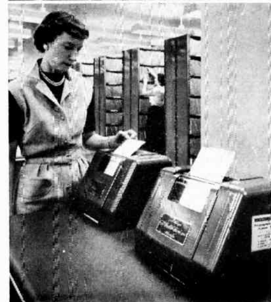
● Top:—The "electronic brain" behind the automatic elevator system. Bottom:—The underwriting department on the fourth floor has to consult permanent record files in the basement and to facilitate the speedy movement of these files, the company has installed a Telautograph service.
