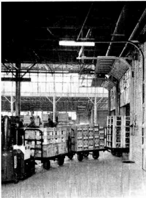
● Guide-O-Matic "operatorless" tractor taking a trailer load of crated goods for shipping.
