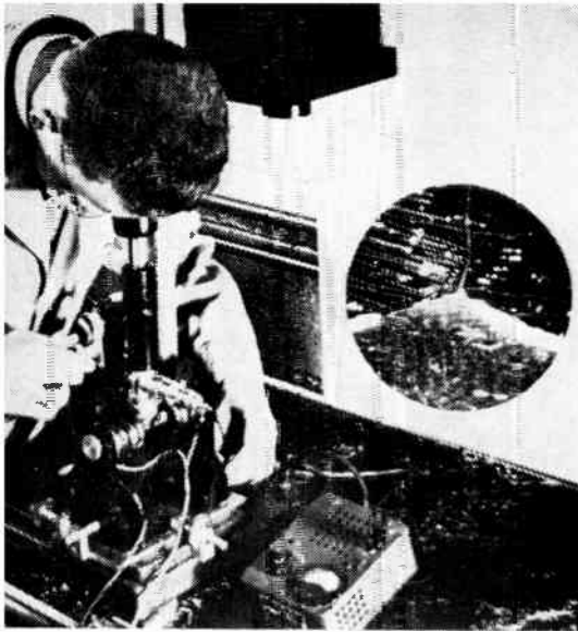
● Peering through the microscope at a prepared sample of electric steel, laboratory technologist, T. G. Nilan studies the formations of magnetic domains within the sample's crystal structure.
