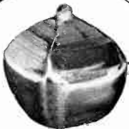
"Single crystal" of pure germanium grown in our plant for use in Junction Transistors.
