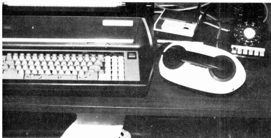
A typical acoustic-coupled modem. There are several disadvantages inherent in these devices, not the least of which is that they take up desk space.
