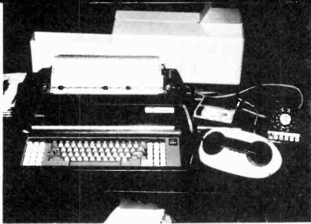
Another way to talk to a computer. A Diablo terminal and modem to communicate via phone lines.
