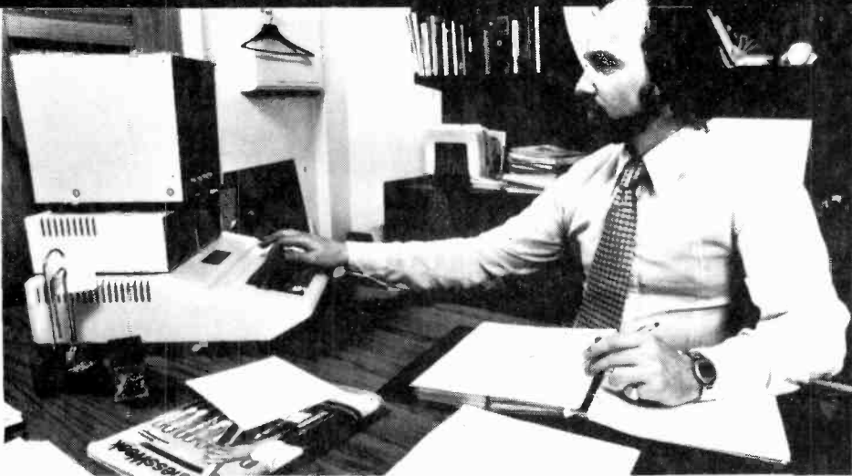
The Apple II business system for offices. Note the two floppy disks under the VDU.
