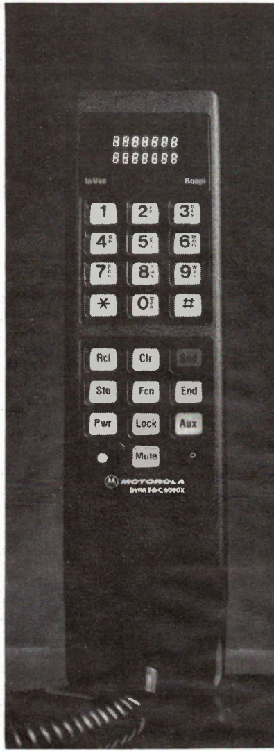
The Motorola 6000X from Bell Cellular has a 32-number memory with a 14-digit review display; other features include incoming call screening and programmable call restrictions.
