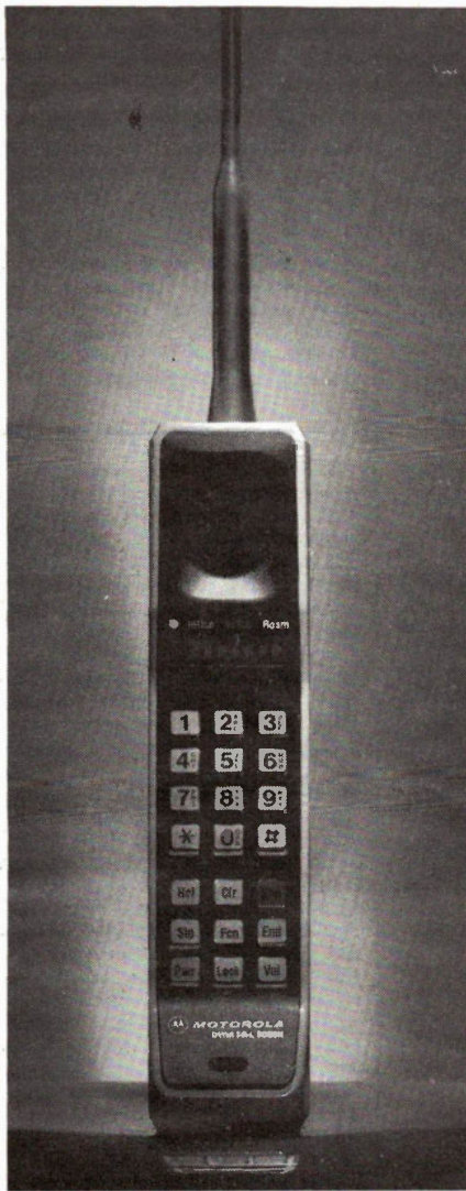
The Motorola 8000X from Cellular is a self-contained portable with rechargeable batteries.
