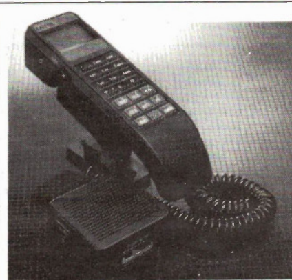
The NovAtel Voyager used by Cantel has a time display, programmable call restriction and connectors for additional handsets or hands-free units.
