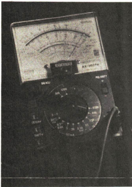
Fig. 6 If the meter pointer does not cross the scale exactly at zero, the meter needs adjusting with the Zero Adjust control.
