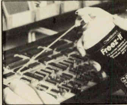
Freez-it from Chemtronics is typical of the many freezing sprays that will restart dead components for troubleshooting.
