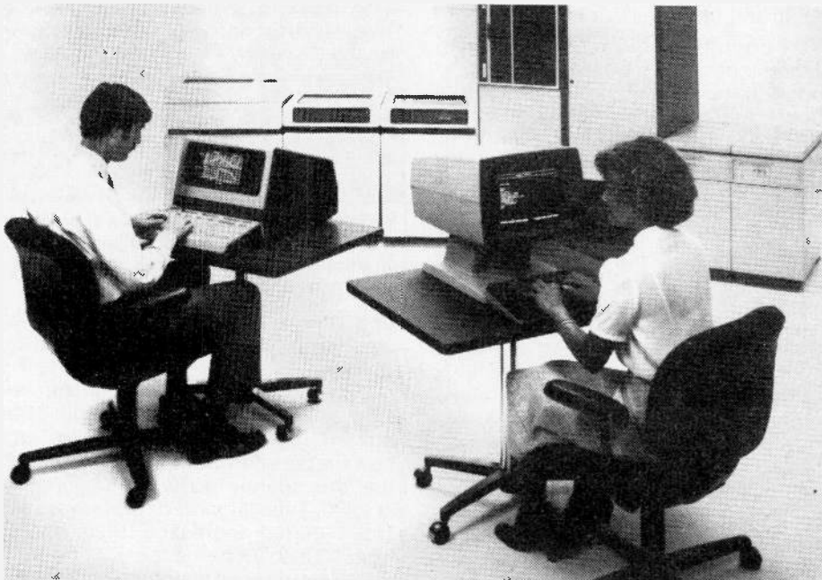
The Hewlett-Packard computers used by the Globe and Mail are similar to Model 65, shown above with optional peripherals. This top-of-the-line model is a high-performance disc-based system with 256K to 2M bytes of memory. The Globe employs eight such units interlinked to provide access to the entire database from any VDT.
