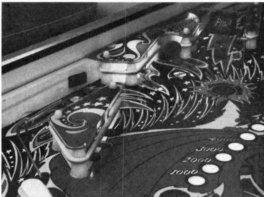
Photo 4. Here target 1 can be seen, and the side alley. The way to cheat is also shown: the two rubber bumpers stuck to the wall of the side alley serve to bounce the ball out of the alley under certain conditions.
