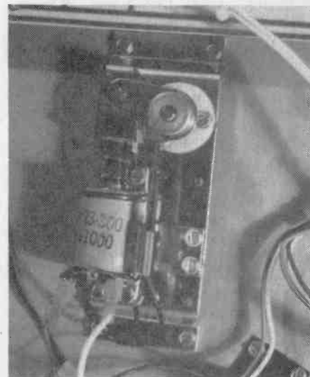
Photo 9. Solenoid for firing the ball off the side bumpers.
