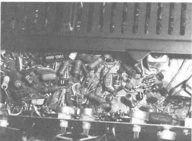
Top: The layout is fairly conventional. Note the convergence panel at the top right. Middle: Accessibility of tube base connections and other circuit points from the top of the chassis is a Zenith feature. (See Techni-Guide for August 1966). Bottom: Some parts of the under-chassis are exposed when the back is removed. The rest is reached by removing a base plate.
