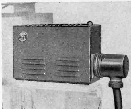
RCA VIDICON TK-21 as used directly on TV projector
