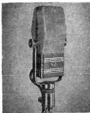
VELOCITY MICROPHONE RCA Type 44-BX
