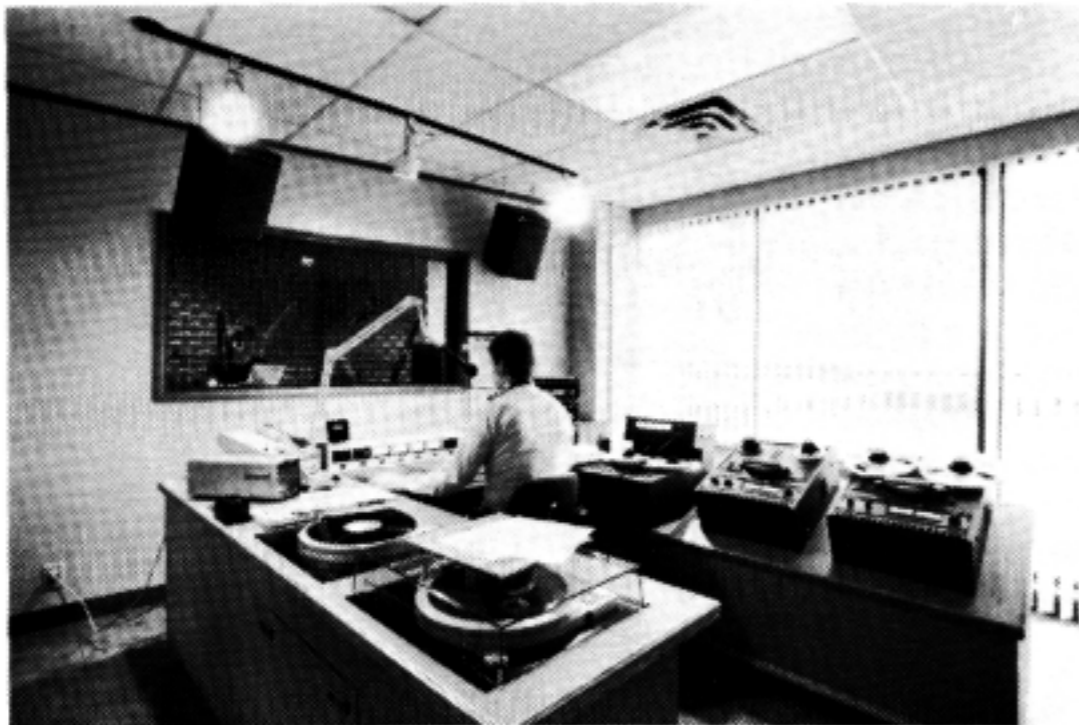
CJOR master control is equipped with Auditratics Series 200 mixing board, ITC cart machines, Otari 5050B tape machines, Technics SP-15 turntables and EV Sentry 100 monitors. Studio equipment includes an Aristocart telephone talk-show system in Studio A, BE 4M50 mixer in news booth.
