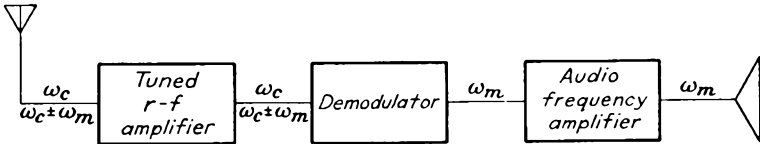
FIG. 1-10. Block diagram of the tuned r-f receiver.
