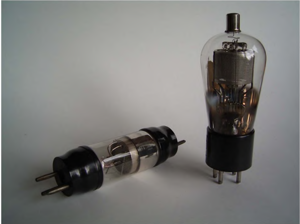
Fig. 8 Screened Valves („Tetrodes“) Left: Marconi-Osram S 625 (thoriated tungsten filament), right: RCA UY224 (indirectly heated cathode)
