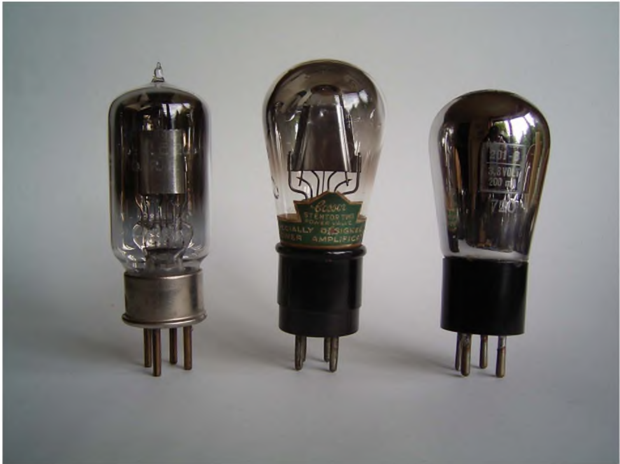
Fig. 7: Output Tubes with Thoriated Tungsten Filament
