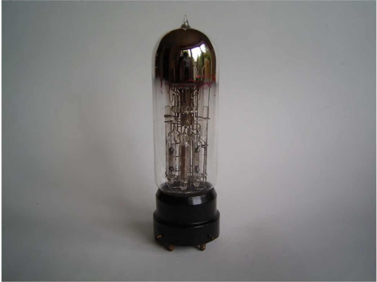
Fig. 16: Multiple Tube 3NF Made by Loewe, containing three tube systems, condensers and resistors
