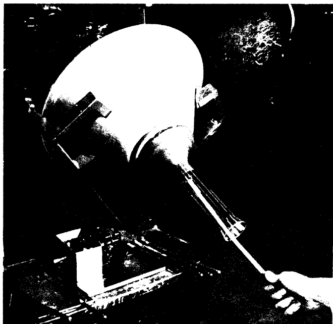
Figure 1. Application of Graphite Internal Conductive Coating
