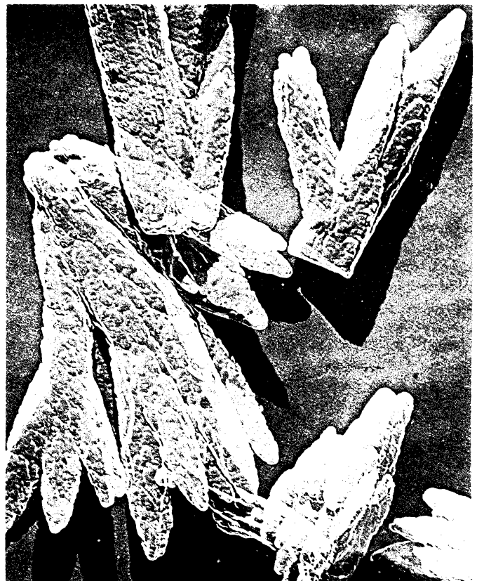
Figure 6. Sodium-Precipitated Triple Carbonate Photographed by Carbon-Replica Technique (electron-microscope magnification x 50,000; courtesy Dr. E. P. Bertin)
