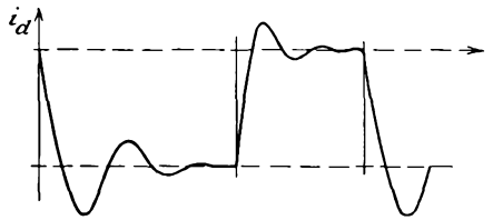
FIG. 21-6. The current in the deflecting-coil circuit when a pulse is applied to the grid of the current tube in Fig. 21-5.
