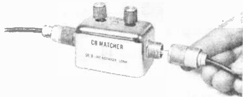
Figure 6. With your rig on, mike button depressed, adjust output loading, tuning controls for highest field, strength reading.
