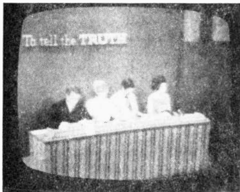
Fig. 20. A snowy picture with little contrast and weak detail is often caused by a weak RF amplifier tube in the tuner. This symptom can also mean a broken lead-in wire, shorted antenna, or open antenna coils.
