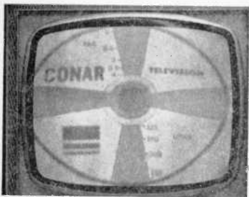
Fig. 20. Condition above is corrected by adjustment of both the horizontal linearity control and the width or drive control.
