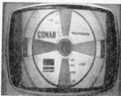
Fig. 21. Picture with insufficient width to fill screen can be corrected by simply adjusting width control until picture is wide enough.
