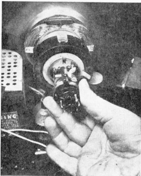
First loosen wing nut, then slide off yoke clamp. (In many sets this will be ion-trap magnet held by a spring around tube neck.)
