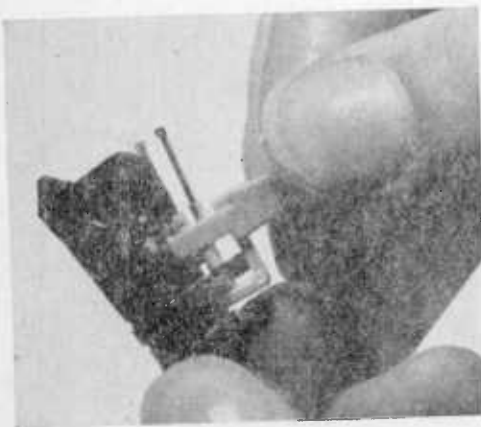
Fig. 8. Gently pull up and away on the stylus assembly; the metal clip gives way with very little pressure.
