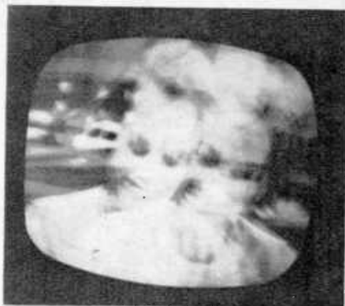
A weird but extremely common trouble occurs when one of the IF tubes makes the picture vibrate.
