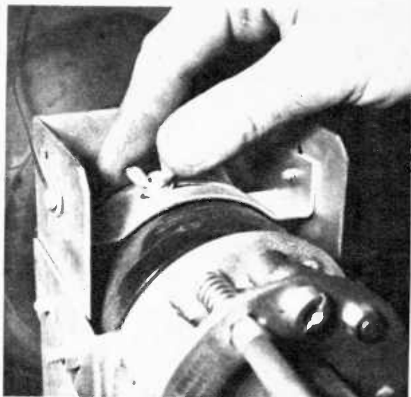
Some yokes have wing nuts on the top of center. Loosen nut and swing yoke for a tilted picture.
