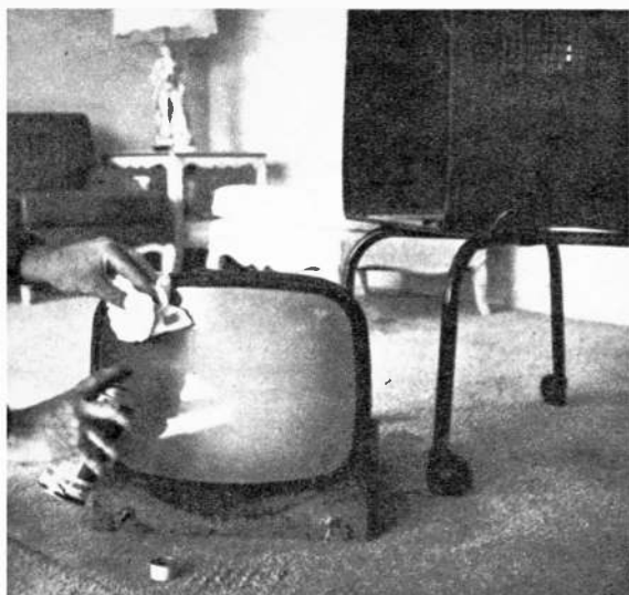
Don't overlook the obvious. A dirty CRT screen can reduce brightness. Pull chassis out and clean.
