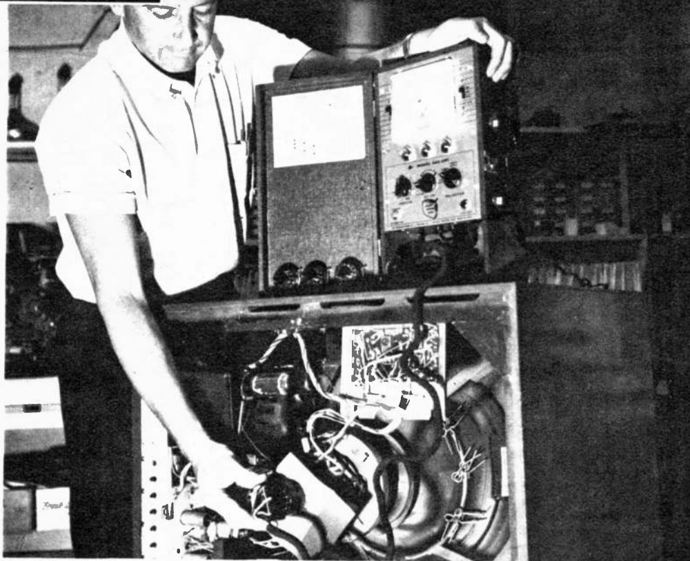
The most efficient way to run a test on a color picture tube is with a cathode ray tube checker.
