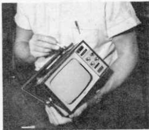
An alternative to substituting for the antenna is to substitute another TV set for the test.
