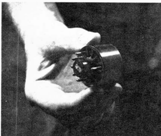
When the plastic socket comes off the neck of the tube you can rethread and solder it back on.
