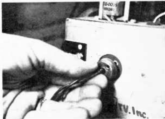
Many TV's have special plugs for speakers. It's designed to kill picture, also, when it's pulled.
