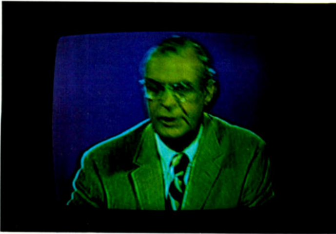
Fig. 24-33 The improper adjustment of the hue control (which is also called the tint control) results in this picture with an overall green shading. This may also be caused by incorrect phasing in the color demodulation circuits. A defect in an automatic tint-control circuit can also produce this general effect. The overall color might also be red or blue, or some intermediate shade.
