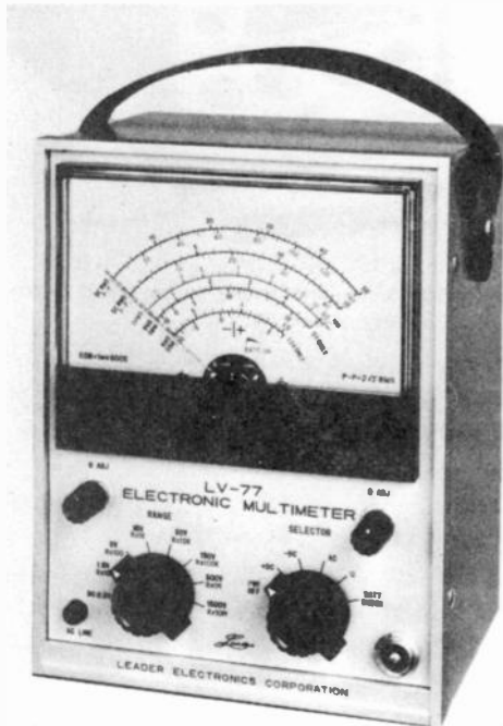
Fig. 23-21. A high-impedance portable FET multimeter. (Courtesy of Leader Electronics Corp.)
