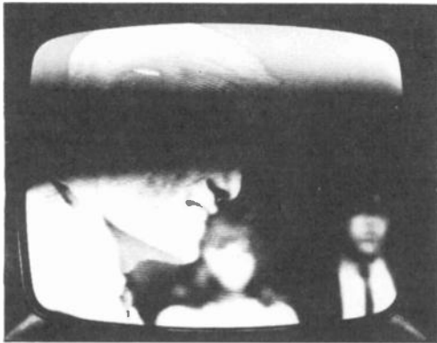
Fig. 12-33. A 60-Hz hum bar in the video signal. If this was caused by a 120-Hz power-supply hum, there would be two dark bars. Note that there is no bending of the picture, indicating that the hum voltage does not affect the sync circuits.
