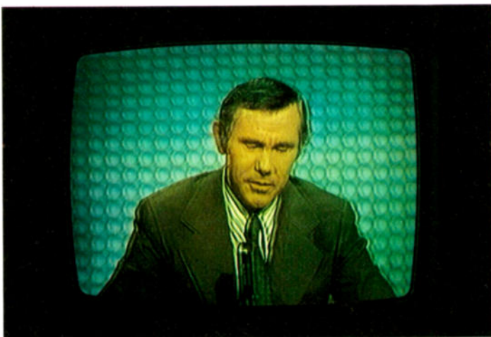
Fig. 24-31 Insufficient color amplitude, which may be the result of an improperly adjusted color amplitude control or a defective bandpass amplifier stage, may result in a weak color display like the one shown here.
