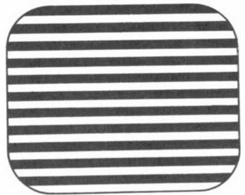
Fig. 24-23. Black-and-white horizontal bars for checking vertical linearity.
