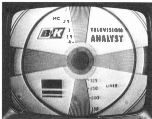
Fig. 12-30. A normal test pattern as displayed on the screen of a typical monochrome-TV set.
