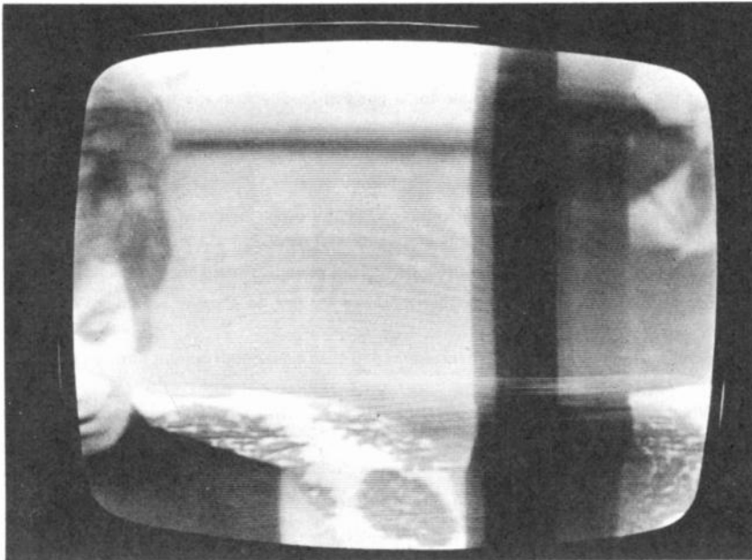
Fig. 17-47. In this picture, the horizontal phasing is incorrect.
