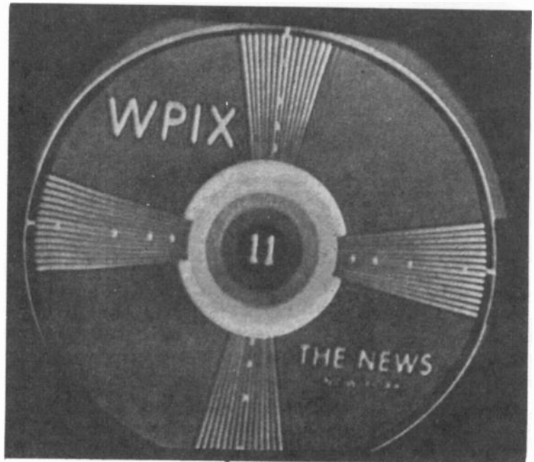
Fig. 24-13. The shadow around the outer edge of the pattern is caused by a deflection yoke which is not as close to the cone of the tube as it will go. (Courtesy Sylvania News.)
