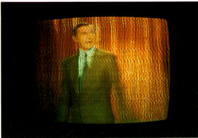
Fig. 24-30 Improper adjustment of the color set fine-tuning control can result in the color sub-carrier beat pattern shown here.
