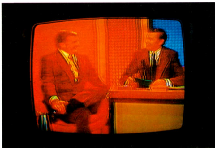
Fig. 24-32 Too much color amplitude will produce a picture with oversaturated colors. An improperly adjusted color amplitude control or a defective automatic color-control circuit may cause this condition.
