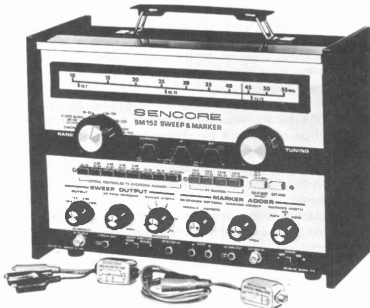
Fig. 23-20. A TV-sweep generator used for monochrome and color sets. All required marker frequencies are available. Post-injection markers are utilized. (Courtesy of Sencore.)
