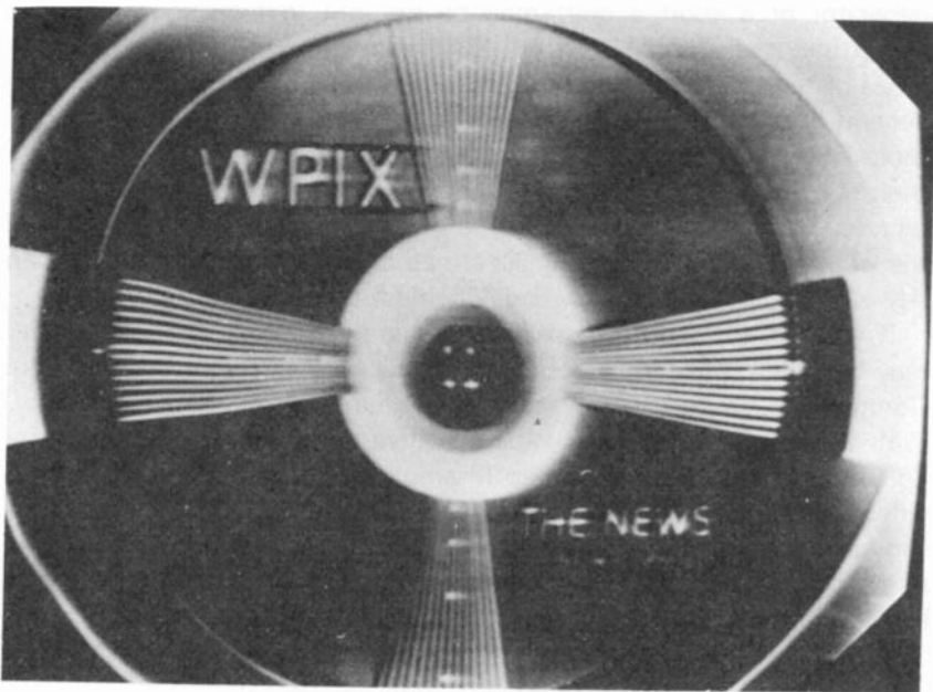
Fig. 24-8. A visual indication of poor low-frequency response in a video system. (Courtesy of RCA.)
