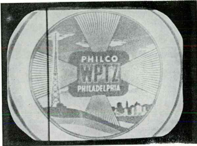
FIG. 16-33. The visual effect of a Barkhausen oscillation.
