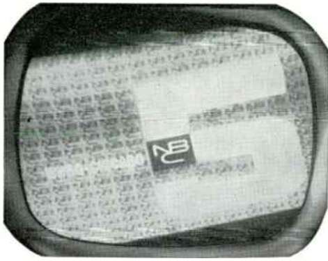
FIG. 9-17. Image incorrectly positioned because of improper placement of deflection yoke.
