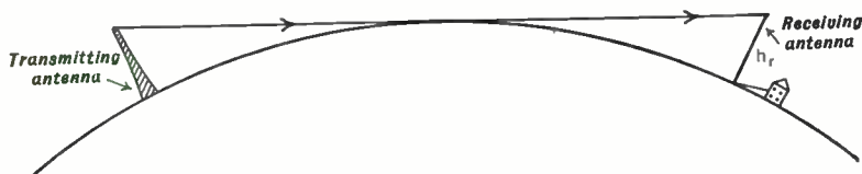
FIG. 2-6. Increase in the line-of-sight distance from the receiving antenna to the transmitter achieved by raising both structures as high as possible.
