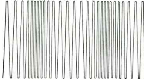
FIG. 14-2. Frequency-modulated wave. The changing spacing between cycles indicates different modulating frequency intensities.
