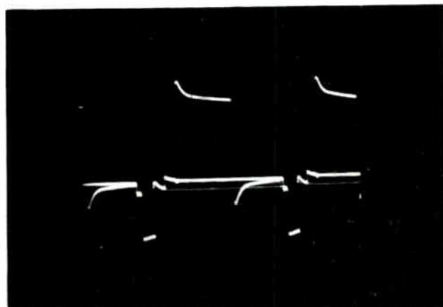
FIG. 76 — NEGATIVE STREAKING — WINDOW SIGNAL — HORIZONTAL
