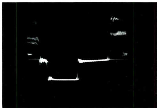
FIG. 94 — RINGING — TEST PATTERN EXPANDED HORIZONTAL
