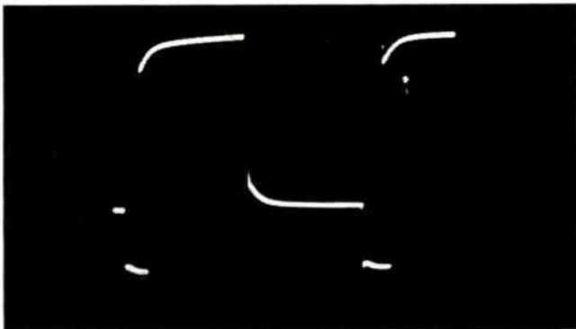
FIG. 70 — WINDOW SIGNAL — LOWS RAISED, HIGHS RAISED — HORIZONTAL
