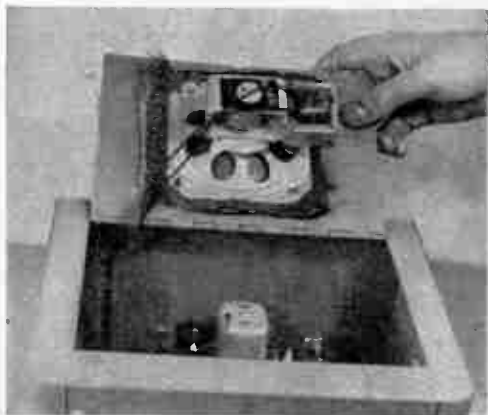
Output is fed into a permanent-magnet loudspeaker (either four or five-inch) set in the cabinet lid
