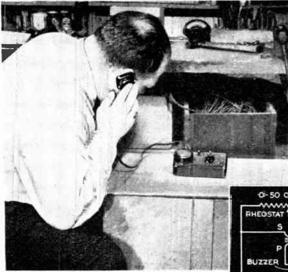
The author using the test circuit shown at the left to measure a small resistor
