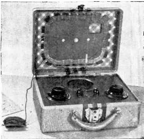
The 9 1/2" by 7 1/2" loop antenna goes inside the lid of the case and can be concealed by paper if desired.
