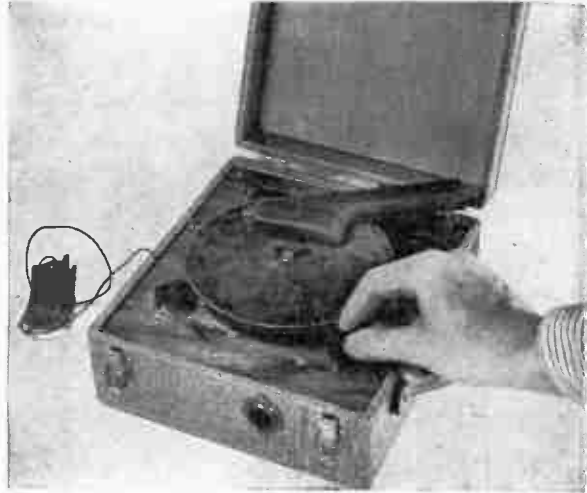
Assembled portable radio phonograph, showing 6" turntable, volume control knobs, and dial
