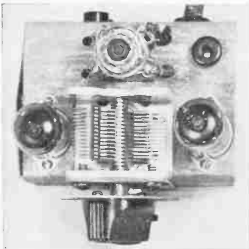
View of the chassis from above. The RF pentode tube is on the right, the rectifier tube at left
