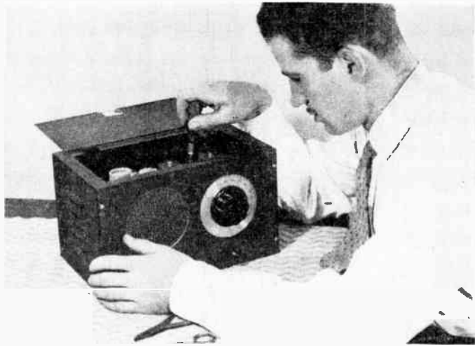
Adjusting the trimmer condensers. The steel cabinet has a hinged lid
