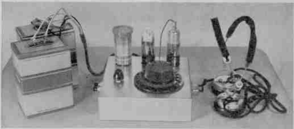
Separate tubes for detection and regeneration give this simple receiver its remarkable efficiency
