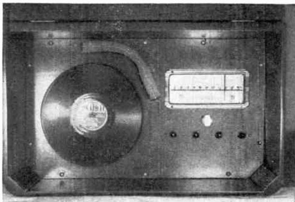
Top view showing phonograph turntable, radio dial, and controls
