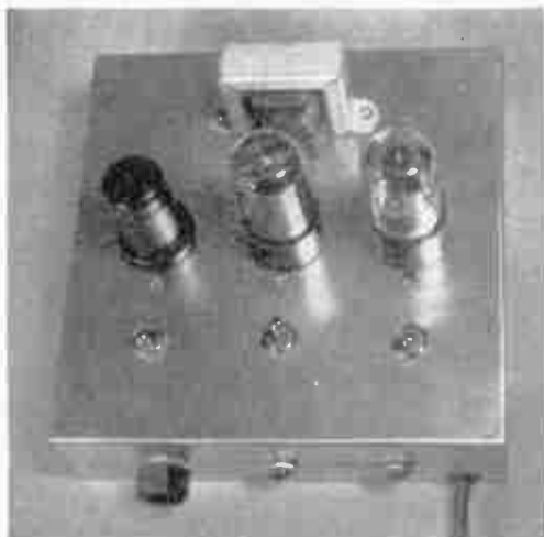
The three tubes, transformer, and control switches as they are mounted conveniently on the top of the chassis before mounting in a corner of the cabinet
