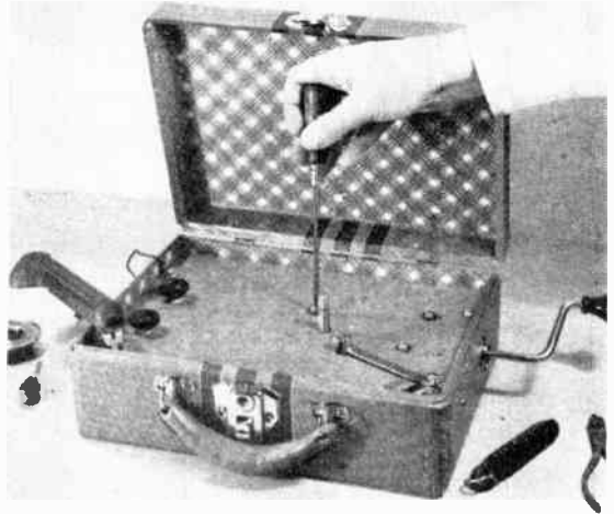
Left, detail of the suitcase, and above, a stage of mounting, before installation of the turntable
