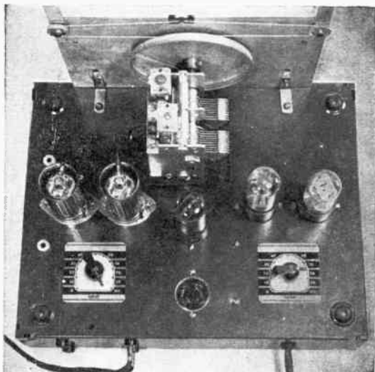
Top and bottom views of the receiver and amplifier. The condenser is roised to be in line with the center of the dial. In the tube bonk, those unshielded are 35Z5-GT/G's. The unshielded coils are shown below
