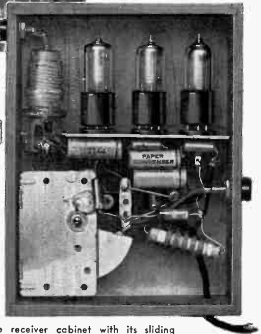
The receiver cabinet with its sliding cover removed to show the three small tubes, tuning condenser, and chassis
