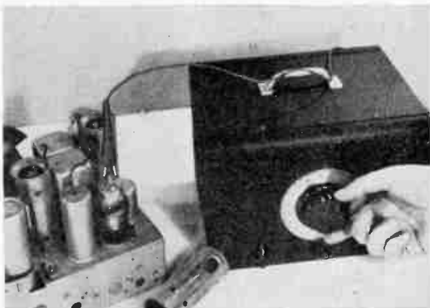
Oscillator shown in use with test prong hooked to screen grid cap
