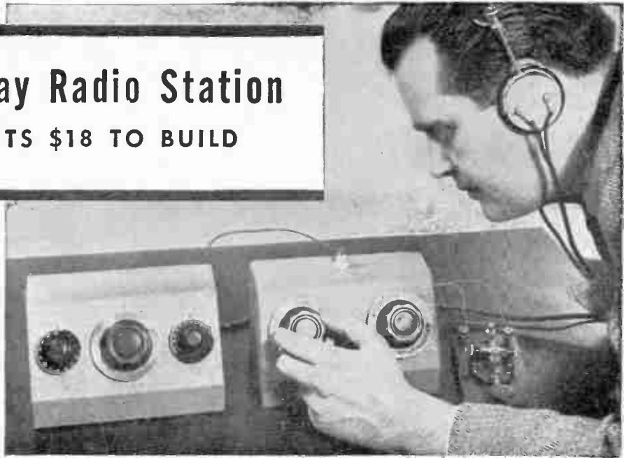
Adjusting the midget transmitter described in this article. Left, the receiver, and right, the sending key
