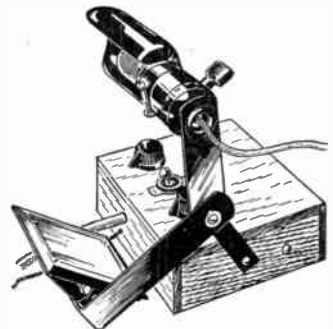
Details of the circuit are shown in diagram. Its tiny 1\frac{1}{2} -volt tube uses a 45-volt "B" battery for plate current
