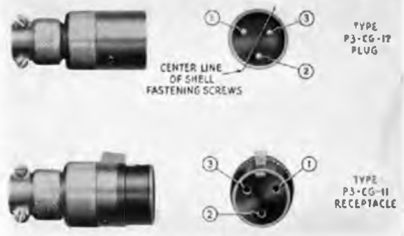
Figure 8—Plugs and Receptacles
