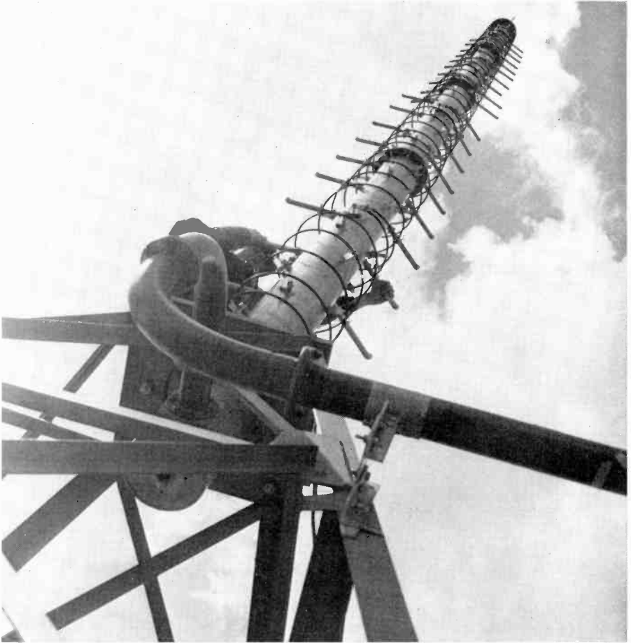
Figure 5.4E. Broadcast television 4-bay UHF high-gain helical transmitting antenna, type TY-24-A, for channels 14 through 19. Courtesy General Electric.
