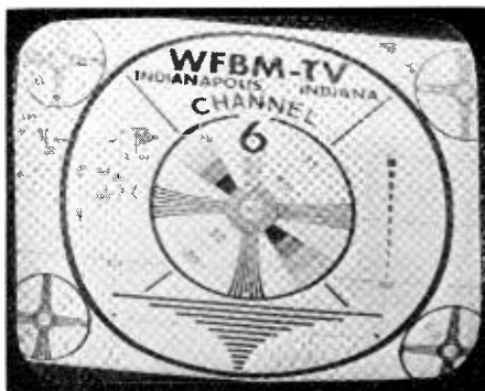
Figure 6.2J. Scanning tilt caused by improper positioning of deflection yoke in camera. Courtesy WFBM-TV.
