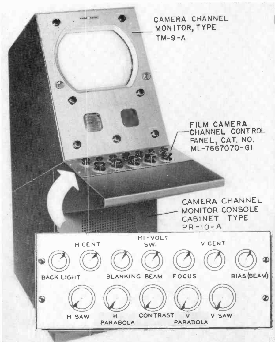
Figure 6.7N. Broadcast television film camera channel control. Courtesy G. E.
