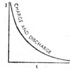
Fig. 55. Current against time for charge and discharge of capacitor.
