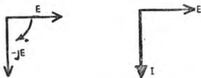
Fig. 39 (Left) and Fig. 40 (Right) show phase relations in an inductor.
