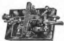
BUG OR SEMI-AUTOMATIC CODE KEY
