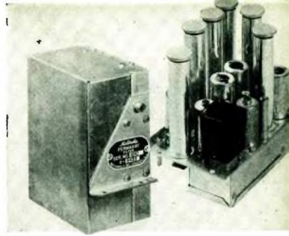
Fig. 5. An IF filter and RF tuner deck
