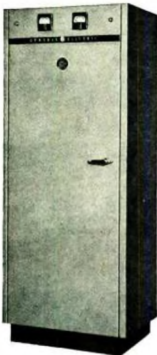
◀ GENERAL ELECTRIC 50 WATT STATION COMBINATION for use in the 25-50 mc or 152-162 mc band. Consists of 50 watt transmitter, receiver, local or remote control terminal equipment and extra space for additional receivers or accessory equipment. Height, 66 inches; width, 24 inches; depth, 20 inches. Designed for "block-building" so that the simple addition of a 250 watt amplifier will boost the power output rating.
