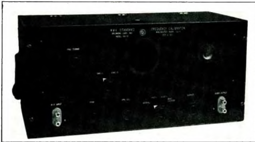
Fig. 26. Circuits are provided for 2.5 and 5 mc., 5 and 10 mc., or 10 and 15 mc.
