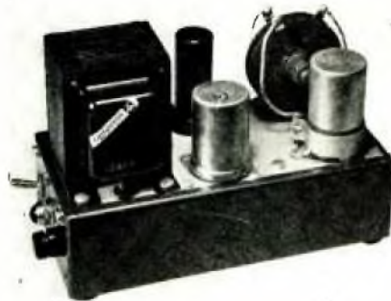
Fig. 11. AC unit for fixed-station decoder
