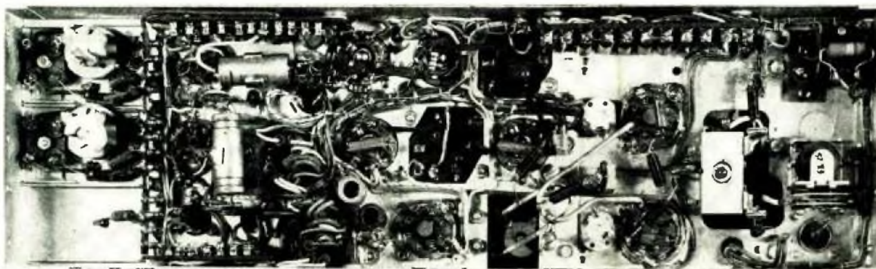
An underside view of the complete 30-watt transmitter section. This illustration should be compared with the views of the chassis and separate decks shown in Fig. 2. The output end of the transmitter is at the right hand side in this view
