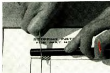
Fig. 33. Cut through to the center wire
