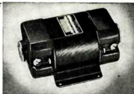
Carter Genemotor 7-1/16" long, 4-1/8" wide, 3-1/2" high. Weight only 10 lbs.
