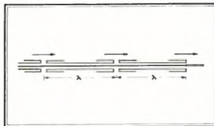
Fig. 19. Instantaneous current in line
