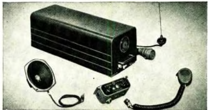
GENERAL ELECTRIC MOBILE COMBINATION MC-201 for dependable operation in the 152-162 mc band. Features single unit design with receiver, transmitter and power supply mounted mechanically on one main chassis. Electrical connection is made instantly through G-E special-design plug-in feature. MC-201 consists of receiver, transmitter, power supply, loud speaker, microphone with retractable cord, antenna, control unit, power and control cables.
