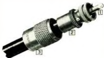
Fig. 32. Be sure that the coupling ring 3 is in place on the cable before the connector shell is soldered to the cable
