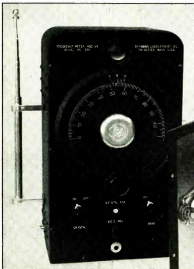
Fig. 20. Browning frequency meter, type S4. Accurate to .002%, it exceeds requirements of FCC.
