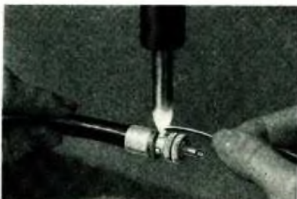
Fig. 39. Solder shell to the cable shield
