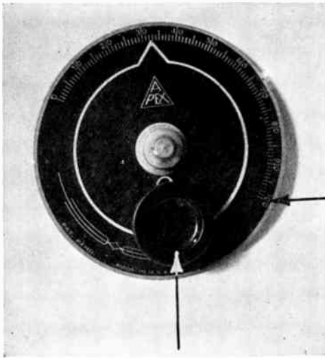
Figure Y: This shows another type of dial used to make very small adjustments on variable condensers.
