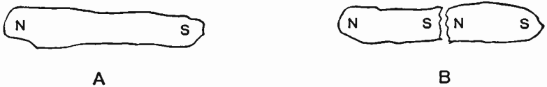
Figure 241. A—Poles on a magnet. B—Arrangement of poles on a magnet broken in half. Note that each piece has two poles.
