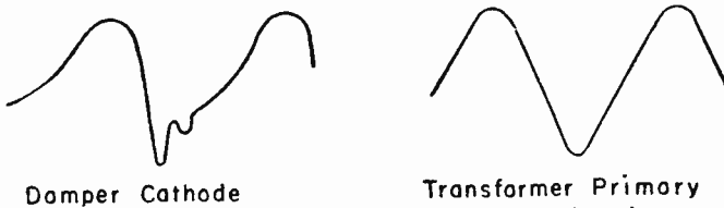
Fig. 22-5.—Current irregularities are smoothed out by the inductor and capacitors of the linearity control.
