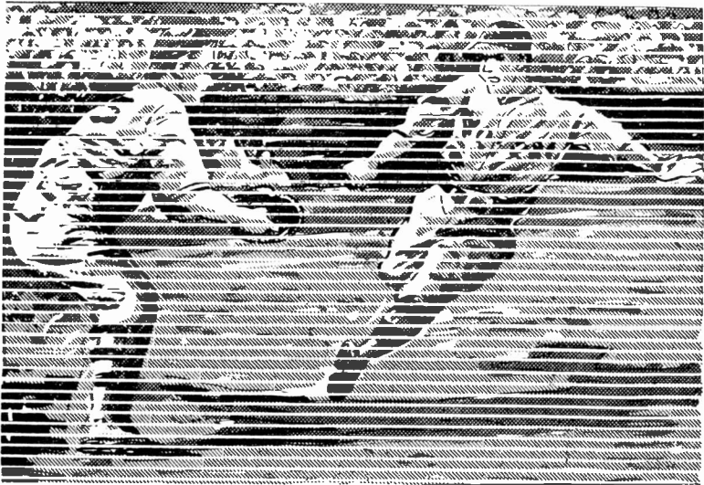
Fig. 114-1.—A picture image is divided into many horizontal lines by scanning.
