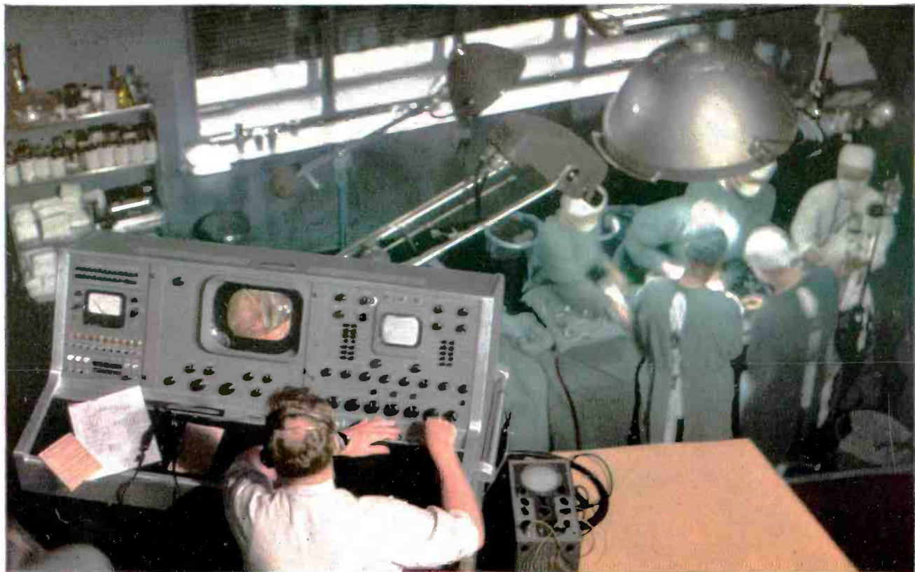
COLOR TELEVISION IN ACTION: Remarkable photo shows one of the recent color television broadcasts of surgical operations at St. Lukes hospital in Chicago. Television camera five feet above patient brought every move of surgeon on 12 x 14 inch color screen. Images were magnified twice life size. Microphone inside surgical jacket enabled surgeon to explain every step in operations. Television receiver in foreground shows picture being received in true colors. These broadcasts done by CBS were viewed by over 4000 surgeons of the American College of Surgeons and were sponsored by Smith, Kline & French Labs. They showed dramatically that color television may become one of the greatest aids to medical education. A complete section on methods of color television (printed in 4 colors) is included in this book.
