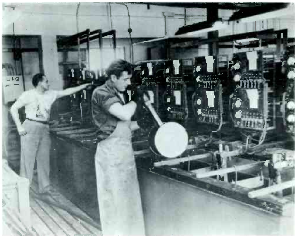
Figure 5-7 From Master To Mother To Stamper
