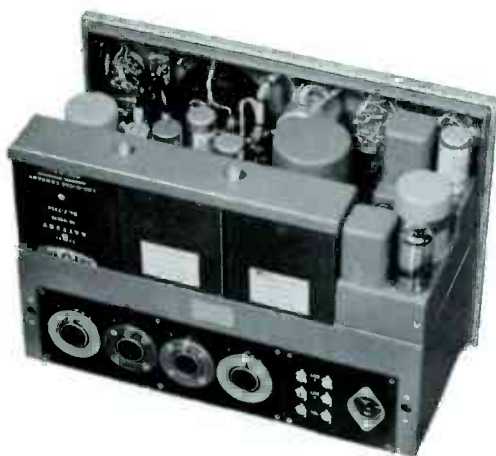
Figure 13-5 Collins Remote Amplifier Back View Courtesy Collins Radio Co.
