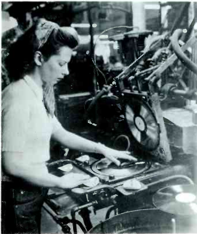
Figure 5-9 Pressing A Record
